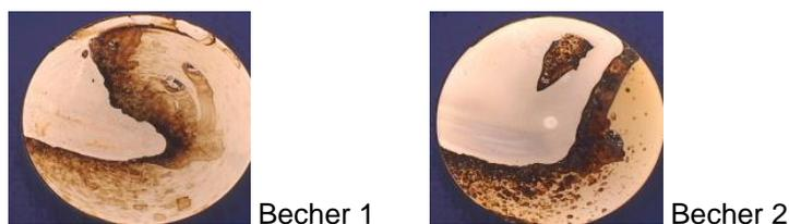
Figure 3 - Comparison of conventional BN100 CLO and CLO using ANM (Coking Bench Test at 310°C)
