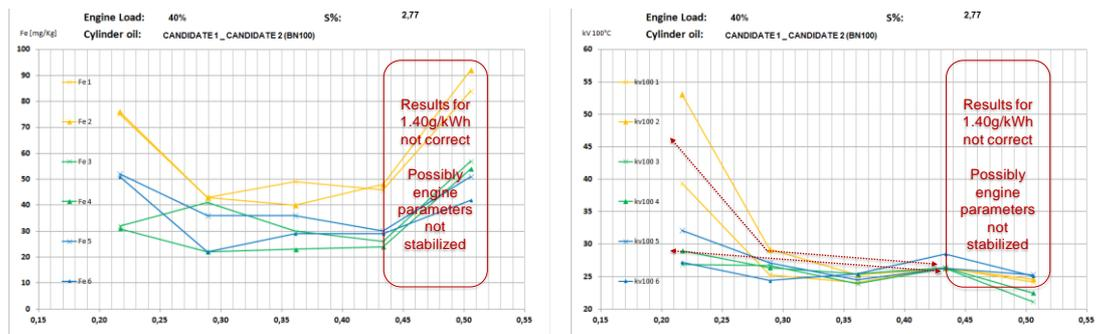
Figure 5 – Fe and KV100 measurement from drain oils (fuel IFO 2.77% sulphur) when changing the ACC factor
