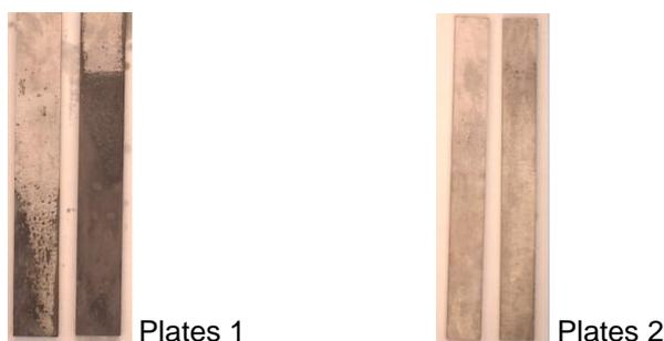
Figure 2 – Plates after corrosion test with conventional CLO and CLO using ANM
