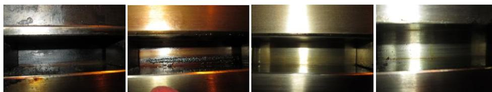
Figure 9 – End of 4420 h test on 14 RT-flex 96C-B engine (piston unit 2)
