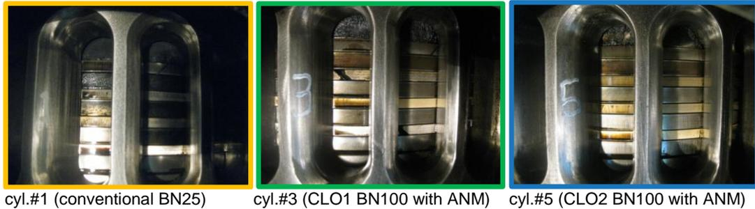
Figure 7 – Ring pack after 200 h test with MDO 0.08% sulphur
