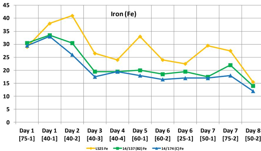
Figure 8 – Fe content from drain oil analysis during 200 h test with MDO 0.08% sulphur
