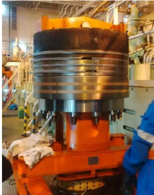
Figure 11 – Piston pulled out at the end of test of TALUSIA OPTIMA in Wärtsilä engine
