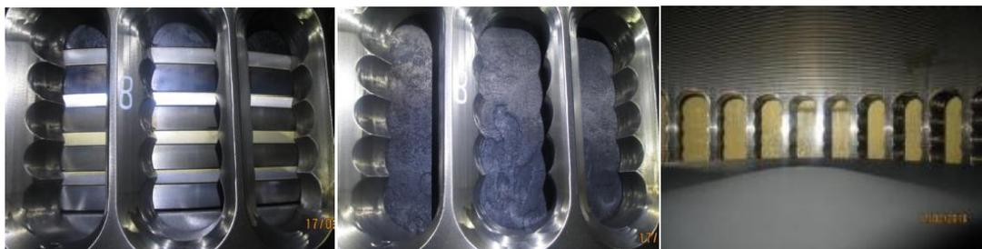
Figure 17 – Statement of one reference cylinder unit (intermediate inspection) during TALUSIA OPTIMA test on MAN engine
