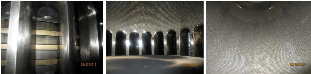
Figure 4 – Test result of BN100 CLO with ANM (fuel HFO 2.77% sulphur) on one cyl. unit
