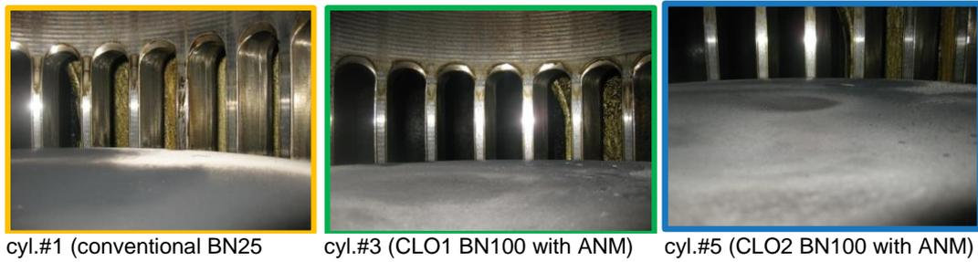
Figure 6 – Piston crown after 200 h test with MDO 0.08% sulphur
